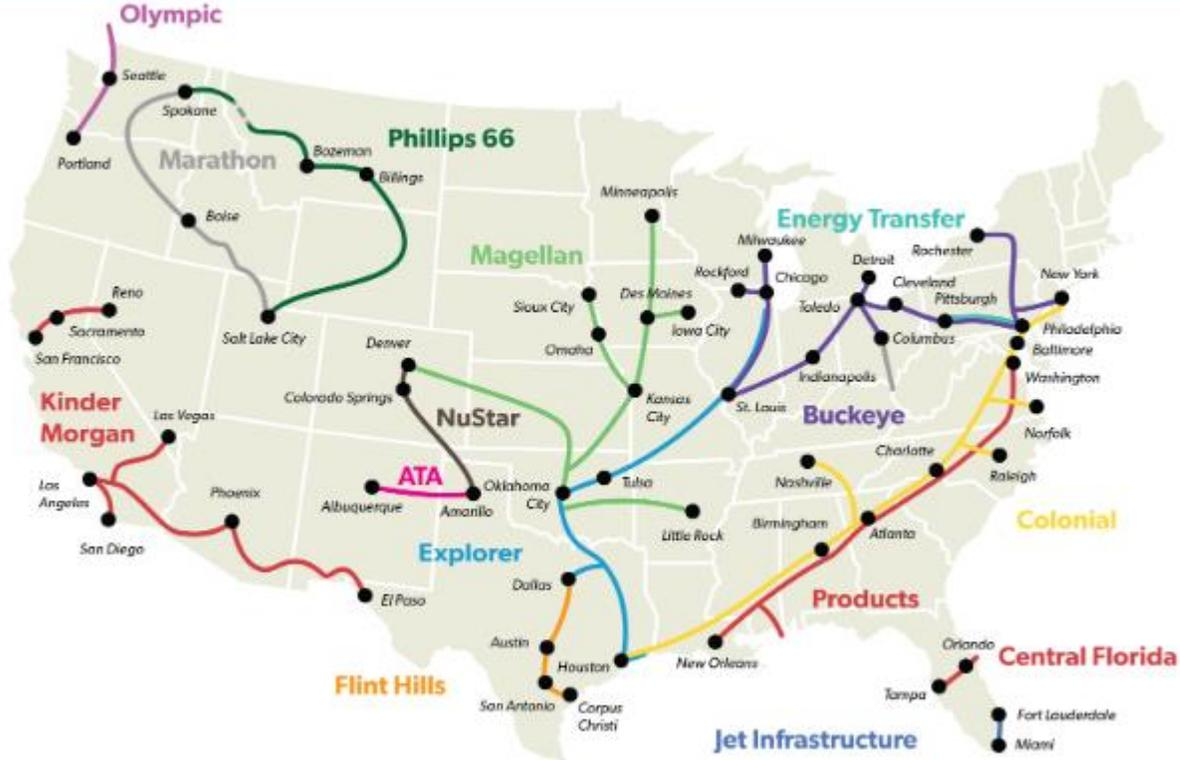
Note: This map provides an overview of the major pipelines in the U.S. that move jet fuel. Smaller pipelines and cities supplied indirectly by pipeline transport are equally important but are not shown on this map.
